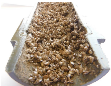
Young zebra mussels in water intake pipe.
